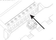
4. Tighten all the seven screws on the Neptune Breakout Box completely
